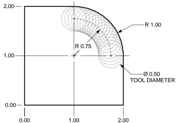
In this example, the center of the radius was entered for the center of the hole pattern. To arrive at the correct hole pattern radius, the tool radius was subtracted from the desired radius. The starting and ending angles of the radius were used as is.
